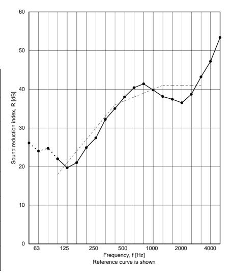
Weighted sound reduction index according to EN ISO 717-1:1996 and EN ISO 717-1 Amendment 1:2006:
